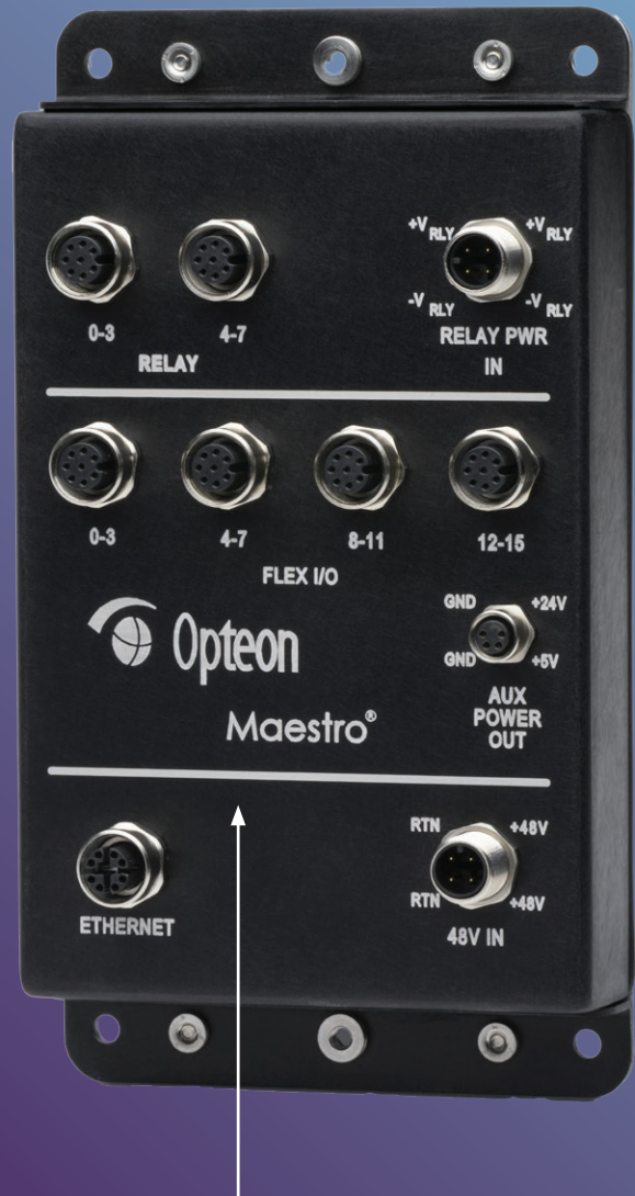
The two horizontal lines marked on the Maestro illustrate the boundaries of the three regions of isolation: PoE/48V, Flex I/O Channels, and Relay Channels.
